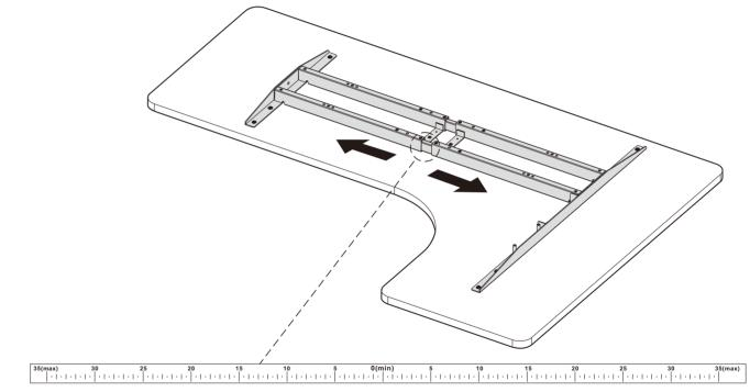
When adjusting the frame position, please make sure it doesn't exceed the range of silk screen printing on the inner crossbar.
