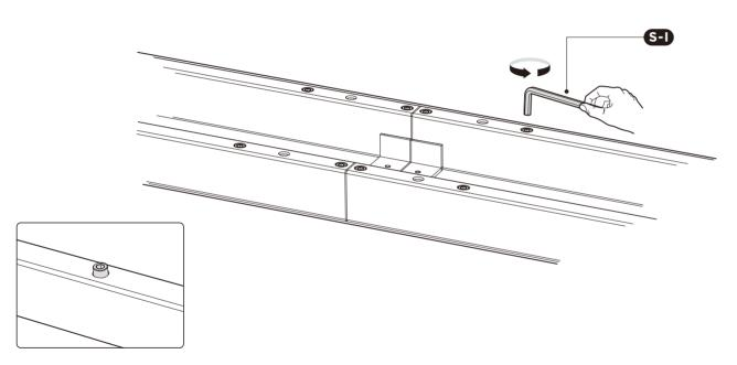
Loosen the hex head screws that fix the adjustable junction, but don't completely take out the screws.
