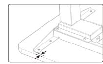
Align the shorter edge of the bracket as close to the desktop edge as possible.
