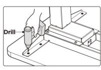
To protect the desktop from splintering or other issues, we recommend drilling pilot holes prior to installing screws.
