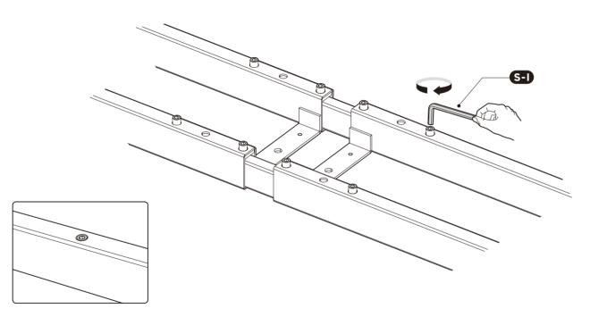
Retighten all the hex head screws to finish the adjustment.
