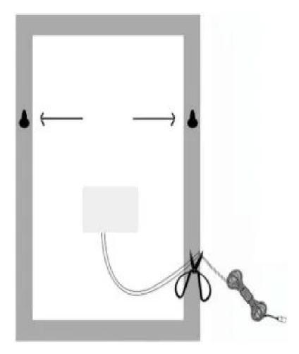
**Electric wiring:** Be sure to leave enough wire to make the proper and safe connection to the Field/Power.
